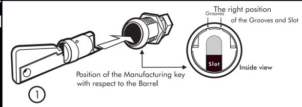
Put Blue Manufacturing key fully into Body (this is locked position of the lock at the door) Think about the position of the Cam, when door will be locked and open. Turn to open position
